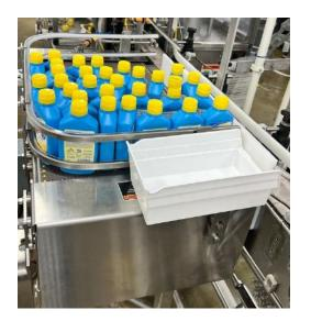
One good example of a yield project is the L22 Capper Rework Table Project by Adam Bauer and Alvin Baker. There was a large amount of yield loss due to Line 22 bottles with crooked/missing caps being kicked off. A conveyor was added to have products smoothly rejected allowing employees to put a cap on, with sanitized gloves, and then put the bottle back on the line. A lexan guard was placed to prevent foreign material contamination.
